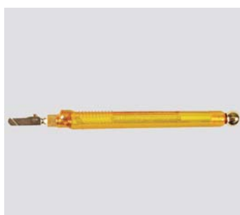
31 281 00 NIKKEN-Glasschneider NC-X02 Carbide-Schneidrädchen, schmal Schneidwinkel 138°, für 2-6 mm Glas NIKKEN glass cutter NC-X02 Carbide wheel, small cutting angle 138°, for 2-6 mm glass
